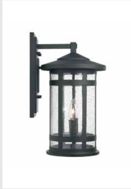
▲ 935521BK WALL LANTERN Black 935521OZ WALL LANTERN Oiled Bronze 9"W x 16.50"H x 10.25"E Backplate: 5"W x 11.50"H x 1"E Ctr/Top: 2.75" Ctr/Btm: 13.75" 2 - 60 Watt E12 Candelabra Antiqued Seeded Glass Wet Rated
