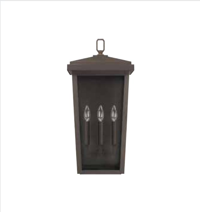
▲ 926232OZ WALL LANTERN Oiled Bronze 926232BK WALL LANTERN Black 11.50"W x 24"H x 8.25"E Backplate: 10"W x 17.75"H x 0.75"E Ctr/Top: 15" Ctr/Btm: 9" 3 - 60 Watt E12 Candelabra Clear Glass Wet Rated
