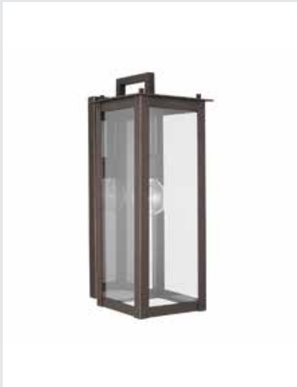
▲ 934612OZ WALL LANTERN Oiled Bronze 934612BK WALL LANTERN Black 8"W x 20.75"H x 10"E Backplate: 5.50"W x 19"H x 1"E Ctr/Top: 11.25" Ctr/Btm: 9.50" 1 - 100 Watt E26 Medium Clear Glass Wet Rated
