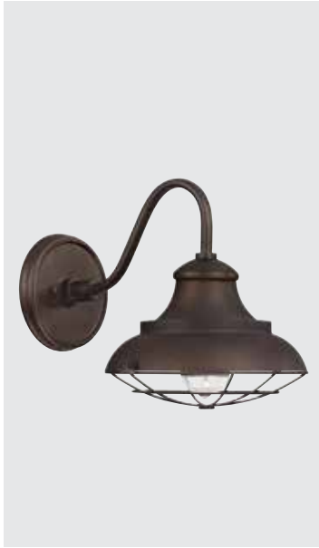
▲ 4561BB WALL LANTERN Burnished Bronze 10.75"W x 10.75"H x 14"E Backplate: 6"W x 6"H x 1"E Ctr/Top: 5" Ctr/Btm: 5.75" 1 - 100 Watt E26 Medium Metal Shade with White Interior Wet Rated
