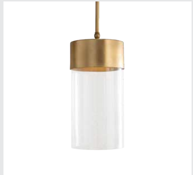
REGAN ▲ 319411CG-437-LD PENDANT Capital Gold 6.50"W x 13.75"H Maximum Hanging Height: 64.25" Includes 6"(1), 12"(1) & 18"(1) Removable Rods 12" Chain; 120" Wire Canopy: 5"W x 0.75"H 1 Board | Lumens: 780 | Color Temperature: 3000 CRI >>90 | Volt/Wattage: 120V 50/60HZ/14W Clear Seeded Glass Dimmable LED
