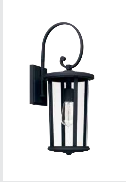
▲ 926711BK WALL LANTERN Black 926711OZ WALL LANTERN Oiled Bronze 8"W x 21"H x 9.75"E Backplate: 5"W x 6"H x 1"E Ctr/Top: 10" Ctr/Btm: 11" 1 - 100 Watt E26 Medium Clear Glass Wet Rated
