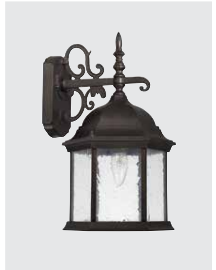
▲ 9833OB WALL LANTERN Old Bronze 9833BK WALL LANTERN Black 9.25"W x 16"H Backplate: 4.50"W x 7"H x 1"E Ctr/Top: 4" Ctr/Btm: 12" 1 - 100 Watt E26 Medium Antiqued Glass Wet Rated
