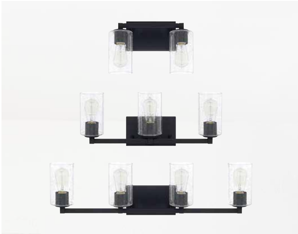
◀ 119821BI-435 VANITY Black Iron 13.25"W x 9.50"H x 5.50"E Backplate: 8.50"W x 5"H x 0.75"E Ctr/Top: 2.50" Ctr/Btm: 7" 2 - 100 Watt E26 Medium Clear Seeded Glass Damp Rated
