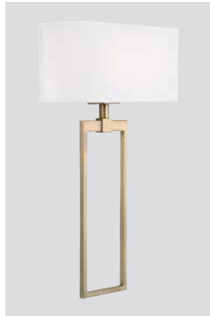
▲ 633321AD SCONCE Aged Brass 15"W x 27.50"H x 6"E Backplate: 14.50"W x 7.25"H x 0.75"E Ctr/Top: 4" Ctr/Btm: 23.50" 2 - 60 Watt E12 Candelabra White Fabric Bolt-On Shade Damp Rated
